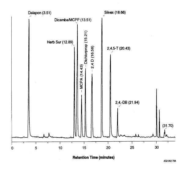
Figure 2. Chromatogram of Herbicides DB-608 Column
