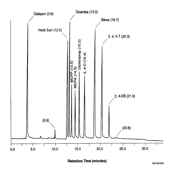
Figure 3. Chromatogram of Herbicides (DB-1701 Column)
