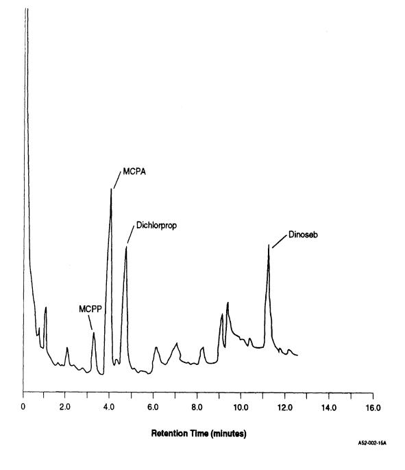
Figure 3. Gas Chromatogram of Methyl Esters of Chlorinated Herbicides on Column 1 (for conditions, see Table 1)
