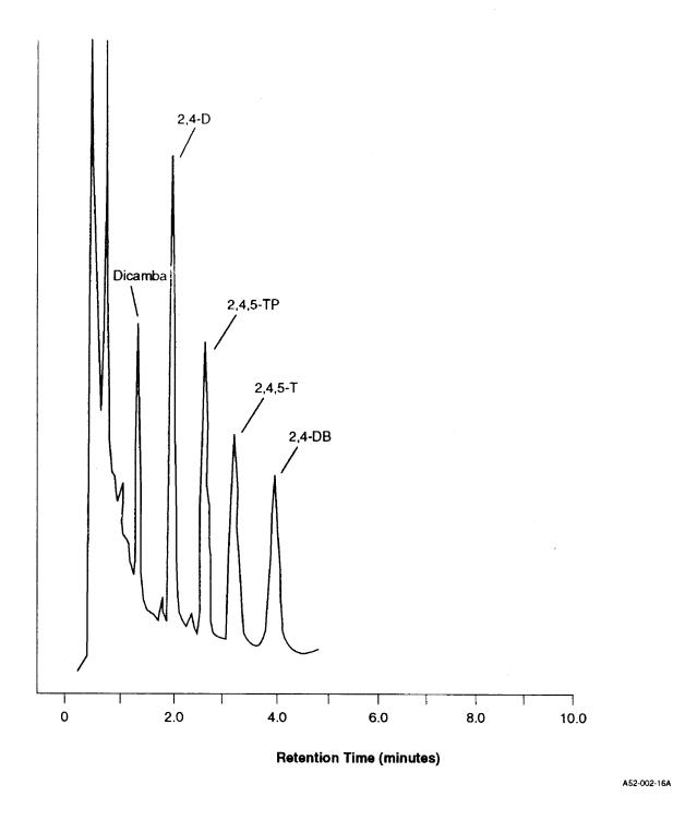
Figure 2. Gas Chromatogram of Methyl Esters of Chlorinated Herbicides on Column 1 (for conditions, see Table 1)
