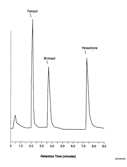
Figure 1. Gas Chromatogram of Organonitrogen Pesticides on Column 1 (for conditions, see Table 1)
