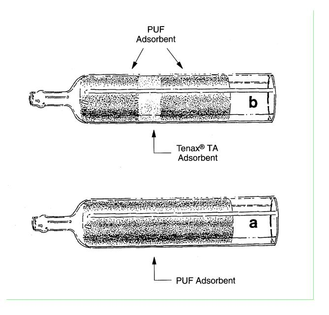
Figure 2. Polyurethane foam (PUF) sampling cartridge (a) and PUF-Tenax® TA "sandwich" sampling cartridge (b).
