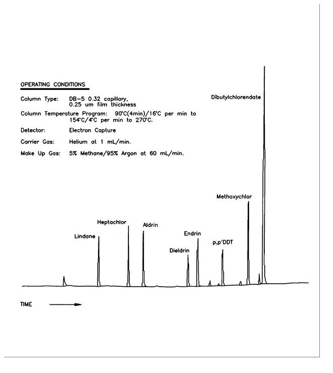
Figure 6. Chromatogram showing a mixture of single component pesticides determined by GC/ECD using a capillary column.
