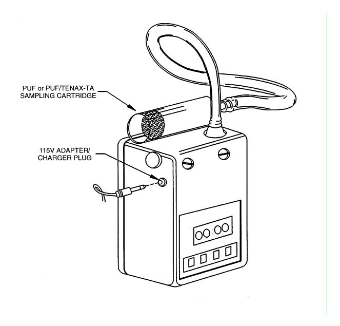
Figure 1. Low volume air sampler.
