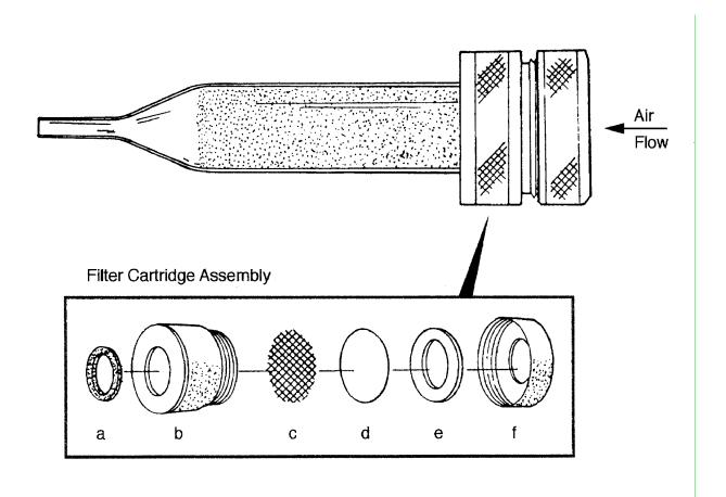
Figure 3. Open-face filter assembly attached to a PUF cartridge:
