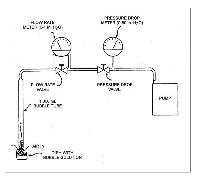
Figure 4. Calibration assembly for air sampler pump.
