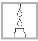
2. Use a pipet to add 0.2 mL of Solution A to the test vial
