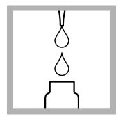
**1.** Use a pipet to add 1.0 mL of sample to the test vial.
