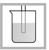
2. Laboratory test: Put the probe in a beaker that contains the solution. Do not let the probe touch the stir bar, bottom or sides of the container. Remove the air bubbles from under the probe tip. Stir the sample at a slow to moderate rate. Field test: Put the probe in the sample. Move the probe up and down to remove bubbles from the probe tip.
